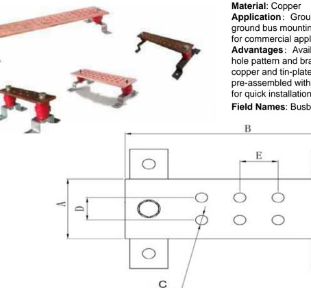
HOLE HOLE HOLE SIZE WIDTH LENGTH DISTANCE DISTANCE THICKNESS HOLE ITEM Std.Pkg. SIZE A SIZE B SIZE C SIZE D SIZE E 20Pcs 6 Holes ZQGB2-6 2" 6" 0.315" 0.79" 1" 1/4" 2" 18 Holes 10Pcs ZQGB2-12 12" 0.315" 0.79" 1" 1/4" 4" 1" 27 Holes 10Pcs ZQGB4-12 12" 0.315" 2.38" 1/4" 1" 63 Holes 4Pcs ZQGB4-24 4" 24" 0.315" 2.38" 1/4"
